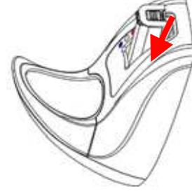
Insert the battery in front of the base to charge your battery with the power adaptor connected. When charging, the base charging LED will be RED. When the battery is fully charged, around 4 hours from completely empty battery, the LED will be solid GREEN.
